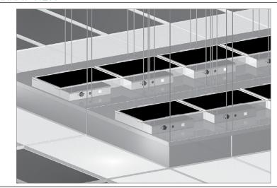
NOTES: Shown left is a typical installation of multiple fan filter units mounted above the service area, completely blanketing the critical area with clean, filtered supply air. For spot applications, a single fan filter unit can be mounted over a work bench or table to reduce particulate counts.
